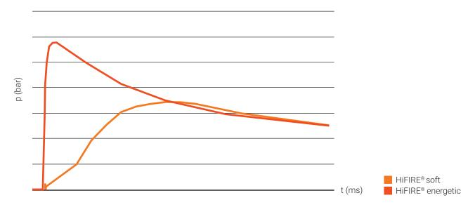
The reactivity of pyrotechnics can be adjusted from extremely high to very moderate, depending on the installation and the intended effect.
