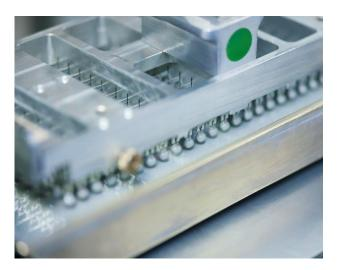
The bridgewire is coated in a primary and secondary reactive high-energy pyrotechnic composition. Specific to each application, special coating systems protect the pyrotechnics from mechanical, chemical and thermal damage, as well as from various environmental effects. The fusehead leg wires can be formed to customer requirement and connected to the application by crimping, soldering or welding.
