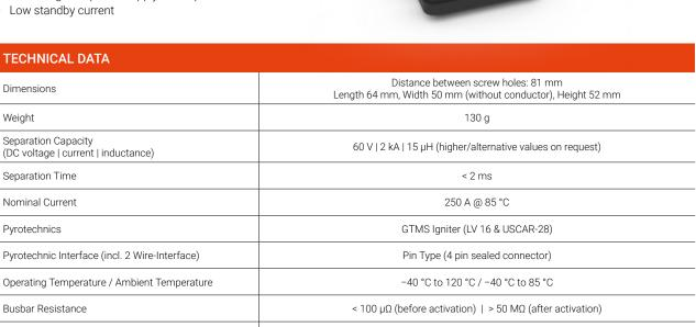
> 50 MΩ (before and after activation) in accordance with LV 124
